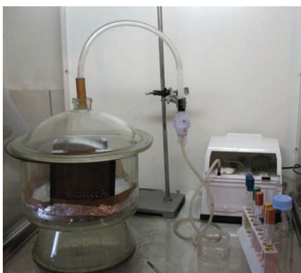
Figure 3: Aerosol chamber used in trial 3 for treatment of mites (in Petri dishes) and bees (in cages provided with metal grid).
